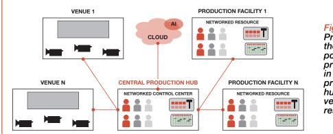
Figure 3 – Distributed Production – venues have the least equipment and staff possible with the crews and main processing equipment residing in the central and distributed production hubs. The production hub can switch between venues to make the best use of resources.
