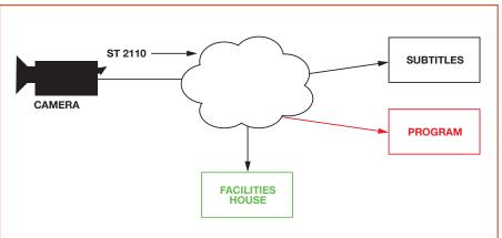
Figure 1 – ST2110 allows us to abstract away the video, audio, and metadata essence from the underlying data link and transport stream. One major advantage of this is that the essence feeds can all be processed independently of each other if required.
