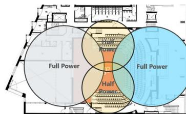
Adding 2 Half Power TCVR's allows for 40 beltpacks on Stage
