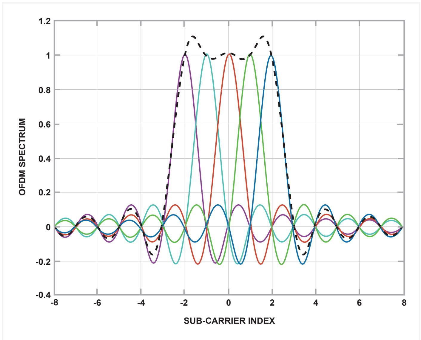
Figure 3 – multiple sub-carriers are brought together so that the peak of one sub-carrier coincides with the null of the adjacent sub-carriers, so interference does not occur. The extent of the sub-carriers forms one channel.
