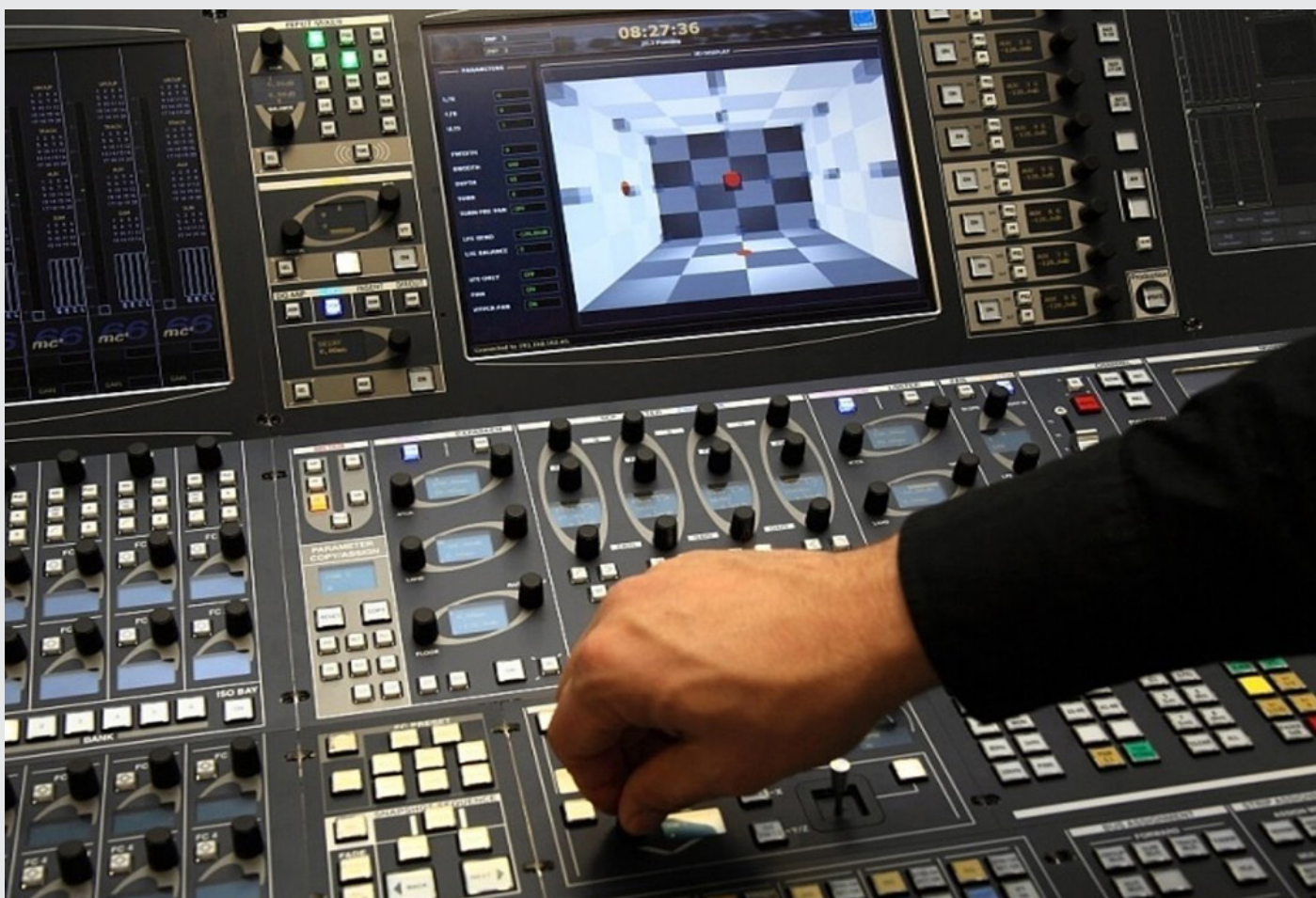
Immersive audio is bringing a whole new panning experience - 3D panning on a Lawo MC 2 66
