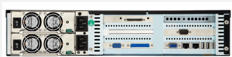
An RTS Trunkmaster acts as the hub for multiple intercoms for Super Bowl coverage. They are networked together using IP.
