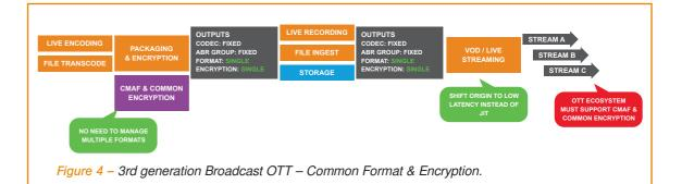
As shown in the grey Outputs boxes, this model produces a set of outputs which are consistent across the delivery chain. There are two drawbacks of this model: 1) it requires an unnecessary amount of central storage (shown with a value of "X") and 2) it creates a pre-formatted VOD library that is inflexible to changes in format type that routinely occur as new consumer devices come to market.
