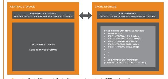
Figure 1 – Central Storage & Cache Storage work together in OTT service delivery.
