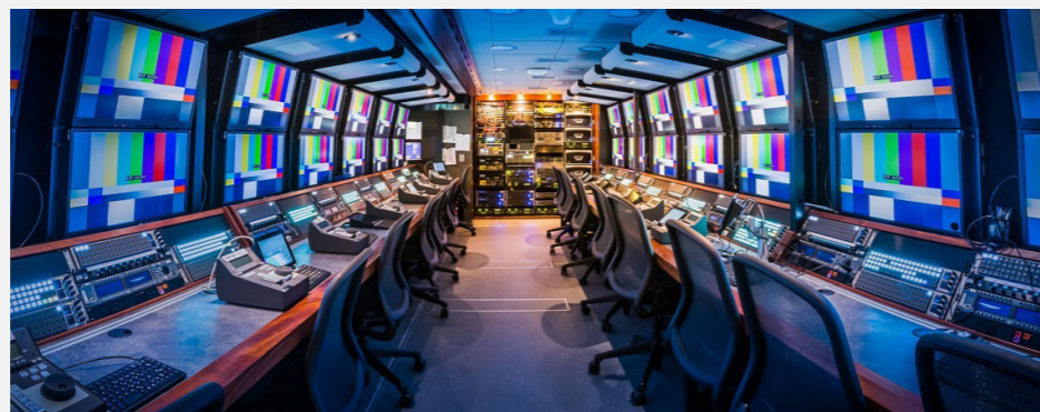
The SSCBS Replay Area inside the C truck includes 20 EVS operators, with two 12-channel XT3 units, four eight-channel XT3 units.
