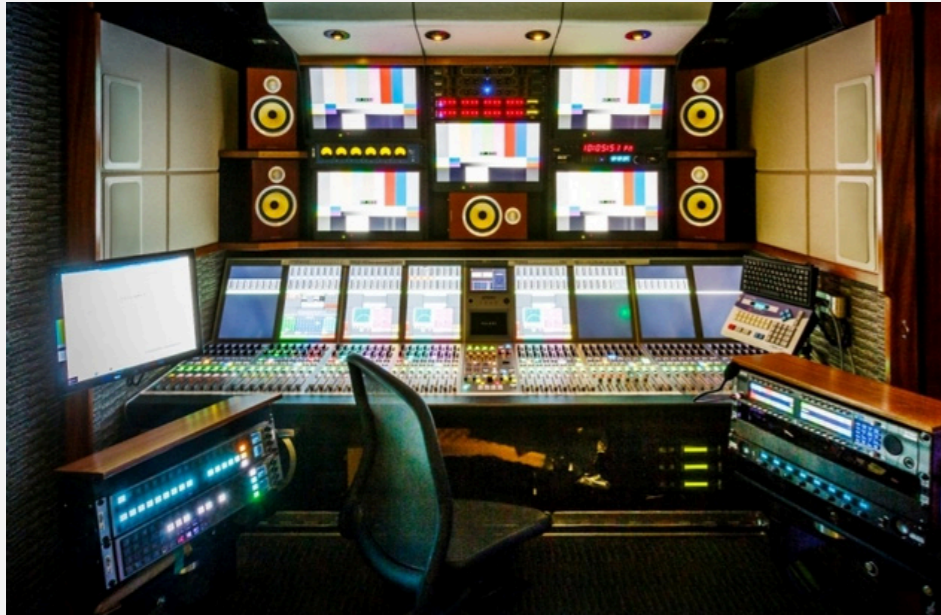
The audio mixing area of the SSCBS A truck features a Dante-networked Calrec Apollo console.
