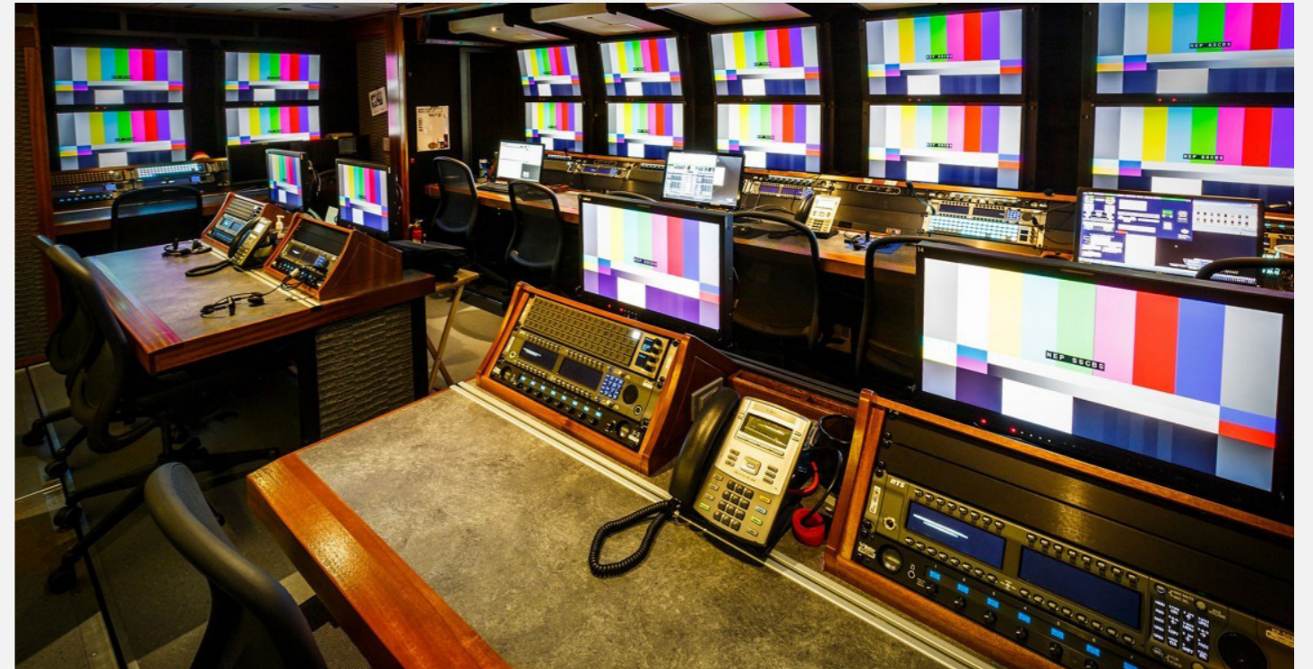
NEP's SSCBS truck, which was used for the NFL regular season, features a wide array of live production equipment, including a Grass Valley Kayenne switcher and multiple EVS XT3 replay servers.
