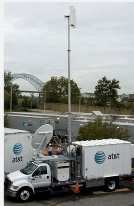
Cellular networks will bring in Cell on Light Trucks (COLTs) and Cell on Wheels (COWs) in anticipation of intense cellular traffic. Photo courtesy ATT.
