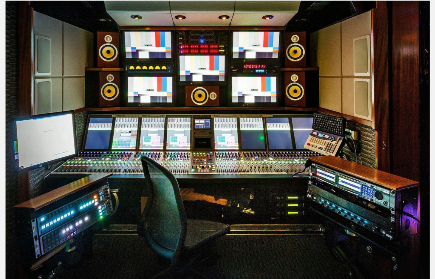
SSCBS audio control room relies on a Calrec Apollo console for main mixing and a Calrec Artemis for tape release.
