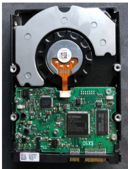
Fig 1 - The underside of this hard disk drive shows the controller PCB with processor, cache memory, and non-volatile memory.
