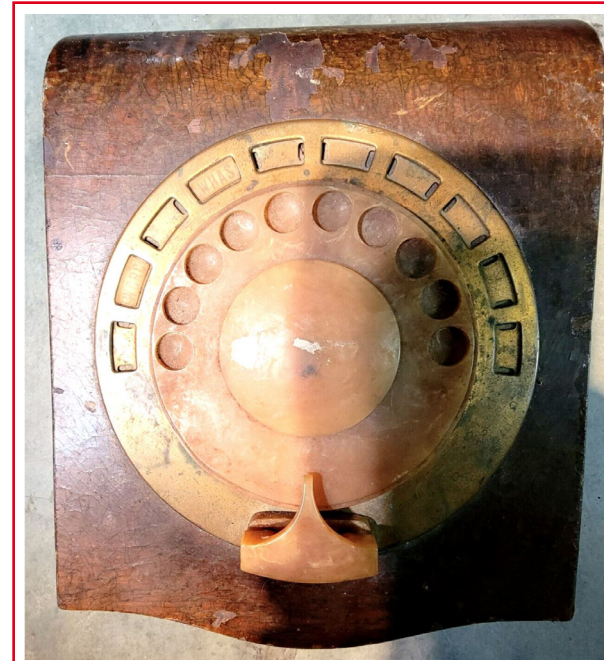
The first, battery-operated, low-frequency, wireless, consumer electronics, remote control radio transmitter was the 1939 Philco Mystery Control.
