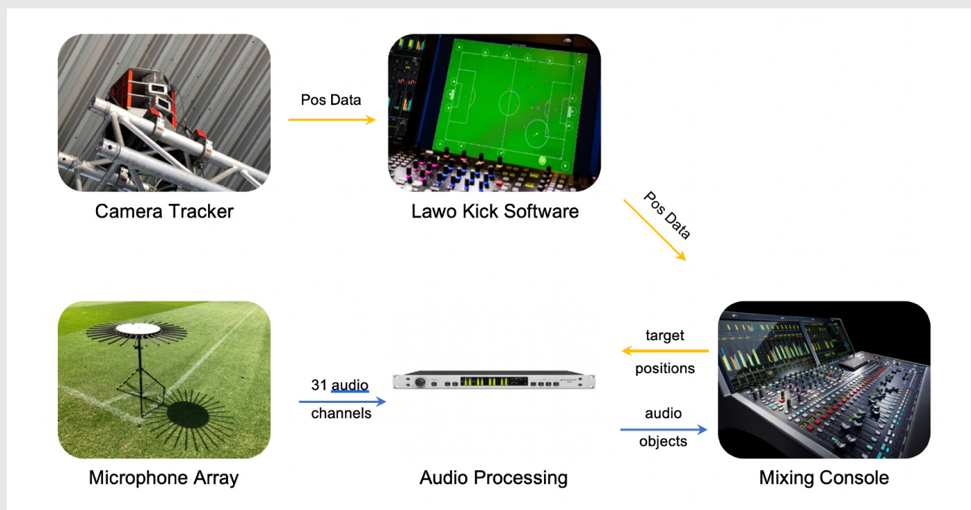
How it fits in - a live broadcast workflow example for the AMBEO Sports Microphone Array, incorporating Lawo's Kick software.
