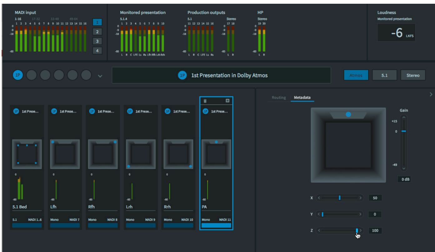
The GUI for Dolby’s DP590 authoring tool showing panning information inside a presentation.
